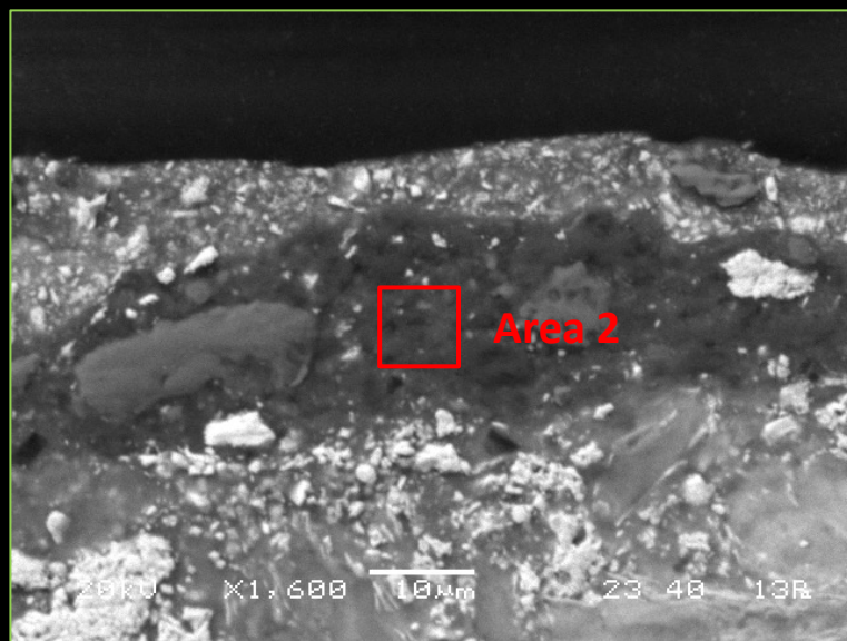
Sample 4 – Cross Section, SEM. Area 2 Microanalysis
