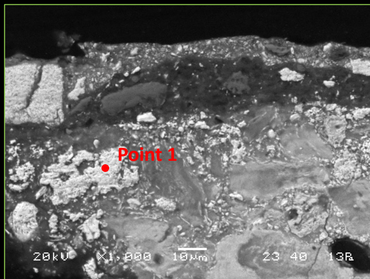
Sample 4 – Cross Section, SEM. Point 1 Microanalysis
