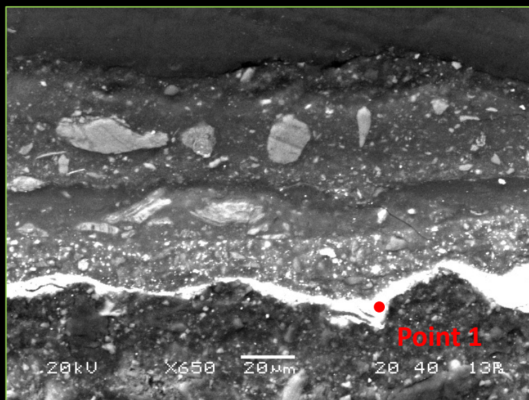
Sample 5 – Cross Section, SEM. Point 1 Microanalysis
